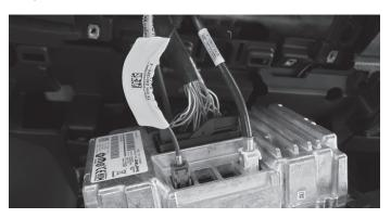
9 The disconnected harnesses from the previous step. These will be used later to connect to the main harness in the installation.
