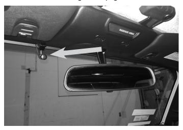
2 Run the Bluetooth microphone cable down the A pillar along the OEM wiring. Route as shown on the diagram on page 12.
