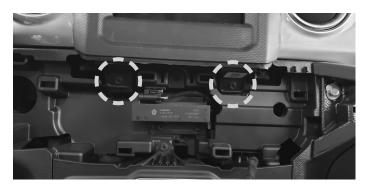
6 This shows where all the OEM clips are at to remove for step 5.
