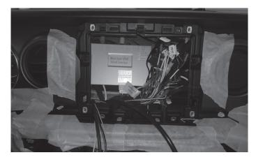
8 Run chime speaker harness from Maestro module to behind the glove box and attach there.
