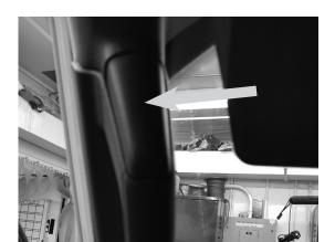
13 Loosen the clips around the top panel visor area.
