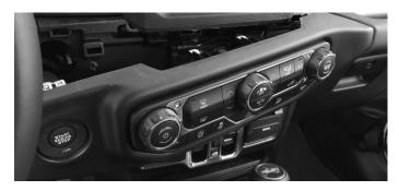
5 Unsnap 6 clips and remove radio bezel using a panel removal tool.
