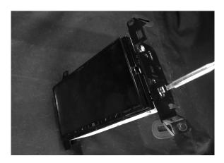
15 Clip in the dash kit and seecure the it using the two screws removed in step 4 of the disassembly. Reinstall the rest of the factory panels to complete the installation.
