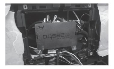
9 Remove the OEM USB from the Center Media panel by unclipping the clips on the sides.
