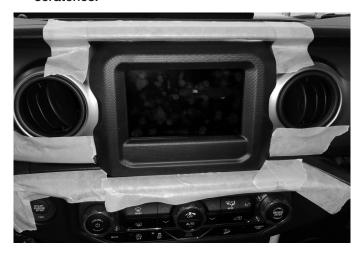
3 Unsnap 10 clips, unplug the 2 harnesses, and remove HVAC panel using a panel removal tool.
