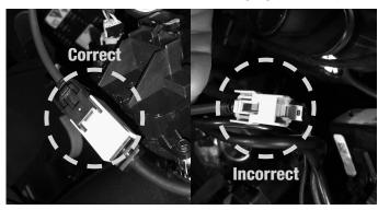
14 Connect the main harness, microphone, USB, HDMI, FM adapter, and other harnesses to the iLX-407 head unit and secure them. Mount the head unit to the dash using the (4) OEM screws removed in step 9 of the disassembly.
