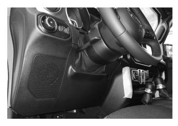
4 Use #2 Phillips Screwdriver to extract (2) screws from the bottom of the radio bezel.
