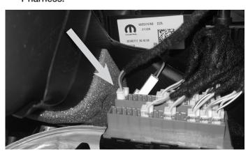
4 At radio cavity, connect the main harness, white FM adapter, and green SiriusXM antenna, and other adapters to factory harness and secure them.
