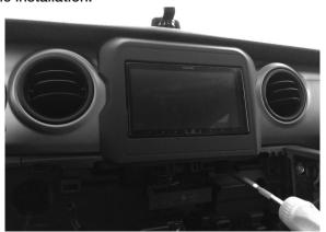
12 WARNING: There are 2 factory micro USB plugs in the dash behind the media center. One is black and one is grey. If the supplied adaptor is plugged into the grey micro USB the factory USB's will not charge. When it is plugged into the black plug all rear USB's can be used for charging (not data).
