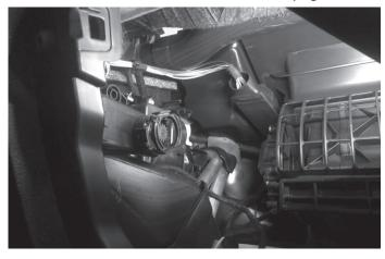
7 Attach the Maestro to the main harness and tuck it in left side of radio cavity.
