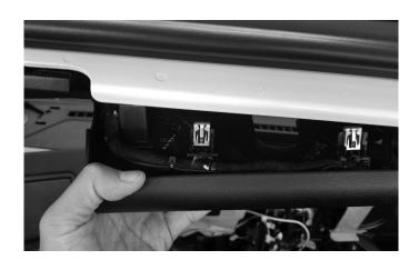
14 Unclip 7 clips and remove the center media stack.
