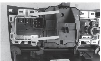
6 Connect the camera interface module to the violet or red factory camera plug and put it in right side of radio cavity. Dip switch 1 will need to be moved down for the Gladiator JT.
