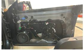
4 Install the new Alpine Speaker & Adapter to the door panel using the factory screws. Plug in green factory speaker adapter plug
