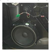
Plug in all remaining factory door connectors. Mount and re-install each factory door panel using (3) T30 Torx. Apply Pressure around the door panel to engage the factory clips. Re-install the Red Reflector Clips
