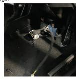
3 Connect Harness "K" black plastic molex end with corresponding plug of CANPRO CP1-S Module "L". Set dipswitch 2 to ON position
