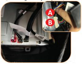
7 Remove the passenger side baseboard lower door trim and locate the connector just before the base of the B-pillar. Transfer the connections to (Plug D)
