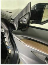
4 Install the new Alpine Tweeter to the housing by positioning the lock tabs and clipping into place.
