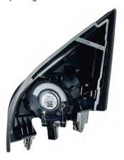
Plug in the original factory connector to the new alpine tweeter and pop the housing into place using downward pressure along the factory clips. Make sure it securely latches into place.
