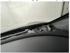
2 Use a Panel Removal Tool around the edge of the dashboard speaker cover panel to release the factory clips. Release the panel and pull upwards to detatch and expose the center stage speakers.
