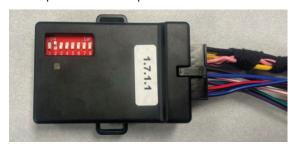
When finished tuck all excess wiring and CANPRO module into the rear center console compartment and re-install the lower cover using factory clips.
