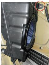
Re-connect the factory subwoofer plug, place the carpet into position and re-install the upper and lower plastic trim panels.
