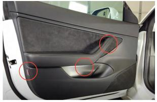
2 Use a Panel Removal Tool around the edge of the panel to release the factory clips. Release the panel and pull upwards to detatch, un-plug the factory panel connections including the green speaker plug. (Note: Some cables are non removable leave the door
