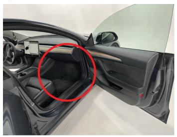
First remove the under dashboard trim panel (#1) by releasing all retaining clips and pulling. After the panel is detached unplug the speaker and footwell light and stow the panel away,
