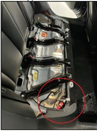
4 Route 12V Power Harness (Plug J) from rear bench seat to the trunk to the amp mounting location.
