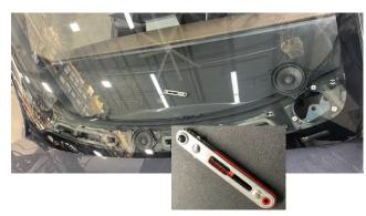
Secure all Alpine speakers to the dash by Re-installing all remaining factory T20 Torx. After speakers are mounted Install the dashboard speaker cover panel by applying uniform pressure to engage the factory clips.
