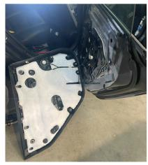
Using hand screw driver nstall the new Alpine Speaker to the door panel using the (6) supplied phillips tapping screws & Plug in the speaker connector
