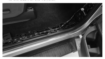
21 Use a utility knife to cut a small incision in the middle of the carpet. Run the wires through this.
