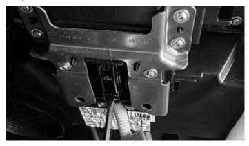
9 Mount the speaker adapter ring using the 3 OEM screws from the previous step. Plug the adapter into the OEM speaker harness. Plug in the woofer terminals. Mount the coaxial speaker to the adapter ring. The adapter ring has pre-drilled holes. It can be attached using 4 of the provided door speaker mounting screws and a phillips screw driver.
