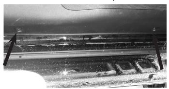
9 Unplug the harness for the door locks, unsnap the door lock button, and release the handle cable. The handle cable has a tab right at the bottom of it that can be released with a flat head screw driver or panel tool.
