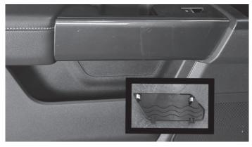
3 Use a panel removal tool to unsnap the top clip and remove the lower reflector.
