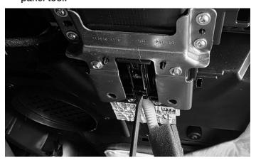
**8** Use a panel removal tool to release the 6 clips along the sides of the panel.
