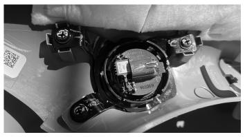
5 Attach the included tweeter mounting ring to the front of the tweeter. This is click and turn in place to hold the tweeter.
