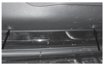
2 Use a ratchet and a 7mm socket to remove the two 7mm screws behind the panel.
