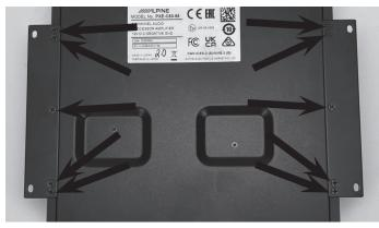
10 Align the front cover and trim bars, then install with the supplied M5x20mm screws (x4) with a 4mm hex drive.
