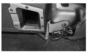
4 Plug in the T-harness to the front and back of the processor. The wire is just can be routed along the passenger side edge of the processor under the tabs so it can stay hidden. There will likely be some slack wire for the +12V constant and ground wires. This can be hidden under the carpet now that all of the connections are made. The mounting bolts can now be tightened down with a 10mm socket and ratchet.
