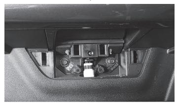
4 Use a ratchet and a 7mm socket to remove the 7mm screw behind the panel.
