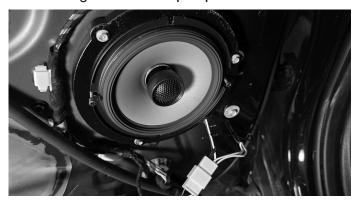
8 Remove the three 7mm screws, unplug, and remove the OEM speaker.
