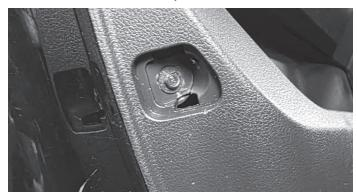
**6** Use a panel removal tool to release the 6 clips along the sides of the panel.
