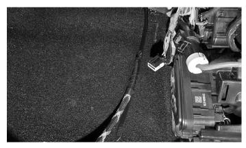
16 Use a wire fishing tool to get from the glove box area to the back of the head unit. Route the T-Harness to the back of the head unit. Make sure to route the correct end through.
