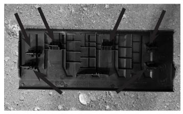
6 Use a panel removal tool to release the 3 clips of the panel below the passenger side dash and remove that. Some trim levels have a module attached to the panel. Remove the two 7mm screws to remove the module and the panel.
