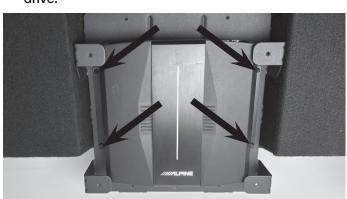
11 The top cover can be aligned to the top of the enclosure and temporarily screwed in. It will need to come off to do the wiring in the vehicle but it's good practice so all the pieces are where they belong.
