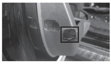
5 Use a ratchet and a 7mm socket to remove the two 7mm screws at the bottom of the panel.
