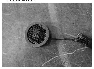
2 Use a ratchet and a 10mm socket to remove the two 10mm screws behind the panel. Remove the panel and unplug the factory tweeter.
