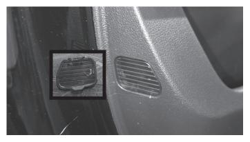
5 Use a panel removal tool to release the 4 clips and remove the top corner panel.
