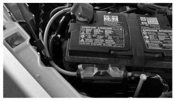
3 Re-connect the negative terminal in the rear and snap the cover back into place.
