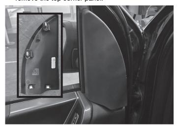
2 Use a ratchet and a 7mm socket to remove the two 7mm screws behind the panel.
