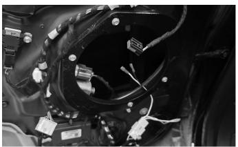
13 Plug in the woofer terminals. Mount the 8" woofer to the adapter ring. The adapter ring has pre-drilled holes. It can be attached using 4 of the provided door speaker mounting screws and a phillips screw driver.
