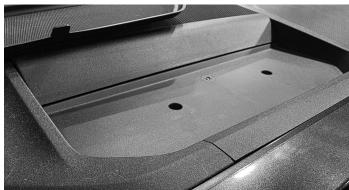
10 Use a ratchet and socket to remove the two 7mm screws holding in the center channel speaker. Unplug that and remove it.
