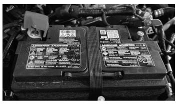
4 Use a ratchet and a 7mm socket to remove the 7mm screw that attaches the ground wire and remove the ground wire and ensure that it can't touch anything.
