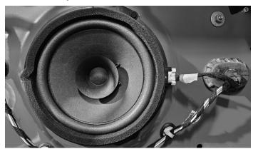
10 Plug all the OEM harnesses back in, mount the door with the OEM clips, and screw in the six 7mm screws to put the door back together. Repeat the process on the passenger side.
