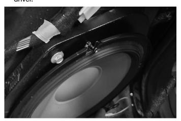
12 Remove the backing from the speaker foam roll and run it along the back outer basket of the 8" woofer.
