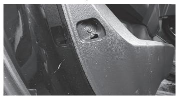
6 Use a ratchet and a 7mm socket to remove the 7mm screw behind the panel.
