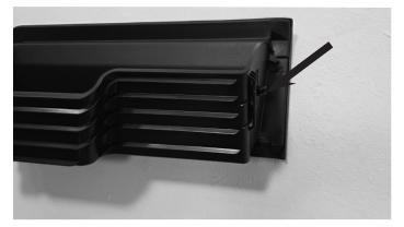
9 This will allow access to the front of the center channel grille cover. Use a panel removal tool to release the 8 clips and remove the panel. These clips can be fairly tight so be careful not to damage the plastic.
