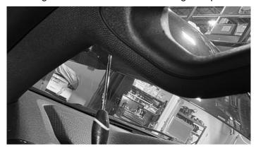
3 Use a phillips screwdriver to remove the 3 factory screws holding the tweeter in place.
