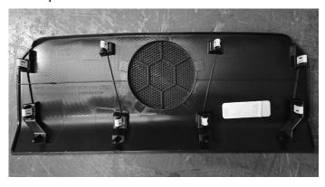
11 Use a panel removal tool release the 10 clips holding in the center channel speaker panel. Again these clips are tight so care will need to be used to remove the panel. This will provide access to the back of the head unit.
