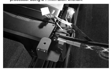
2 The drivers side seat bracket also has a hole in it from the factory. With the passenger side still lose line up the sub enclosure bracket with the factory hole and hand tighten the nut and bolt.
