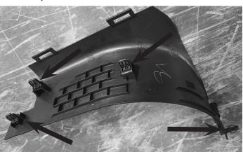
4 Use a panel removal tool to release the clips of the D pillar and remove it.
