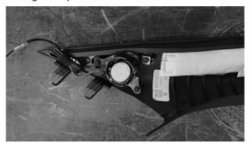
9 Reattach the factory panel and repeat the process for the passenger side.
