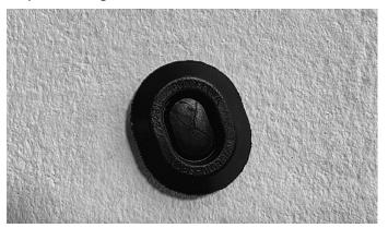
15 With both the wires through remove the tape and run them through the OEM grommet. Snap the grommet back into place on the firewall.
